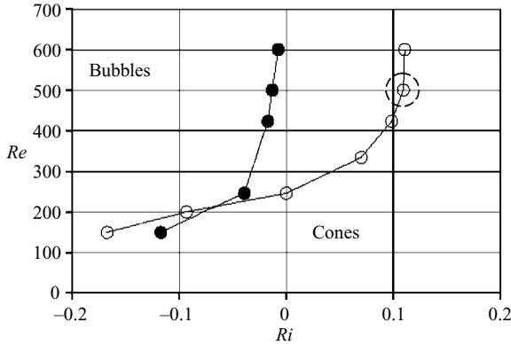
FIGURE 8. The boundary between cone and bubble configurations. Open and filled circles correspond to the IC and IH experimental setups, respectively.
