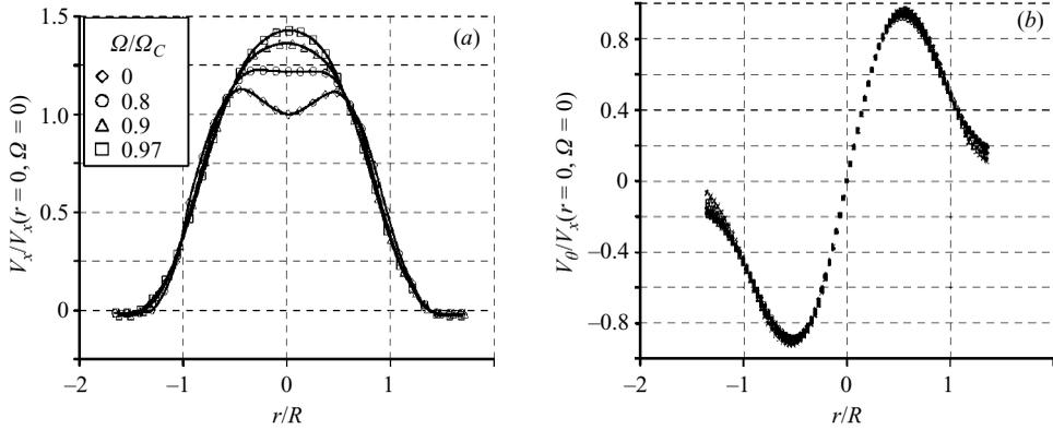
FIGURE 3. Velocity profiles measured at  $x = X_1 = 4$  mm,  $Re = 500$ ,  $Ri = 0$  and normalized by the centreline axial velocity of the corresponding non-swirling jet. (a) Axial velocity profiles at several swirl ratios and (b) azimuthal velocity profiles measured every  $15^\circ$  along the azimuthal coordinate at  $S_{int} = 0.51$ .
