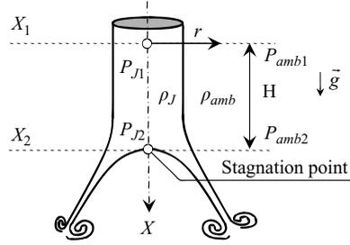
FIGURE 1. Schematic drawing of cone vortex breakdown.
