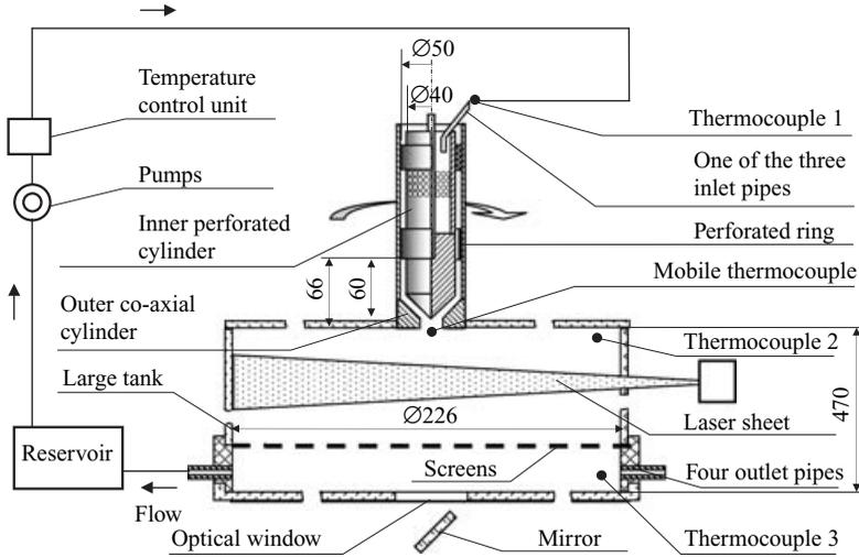
FIGURE 2. Schematic view of experimental apparatus.
